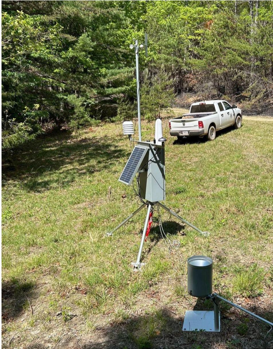
*Figure 21. Photograph of the Eastern Divide Portable RAWS TT386 on the Sinking Creek RX.*
